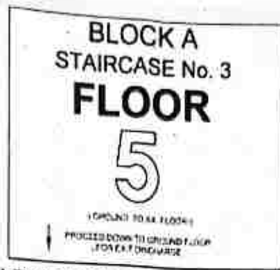
9A EXAMPLE OF A STAIRWAY MARKING SIGN [FLOOR INDICATION BOARD]
